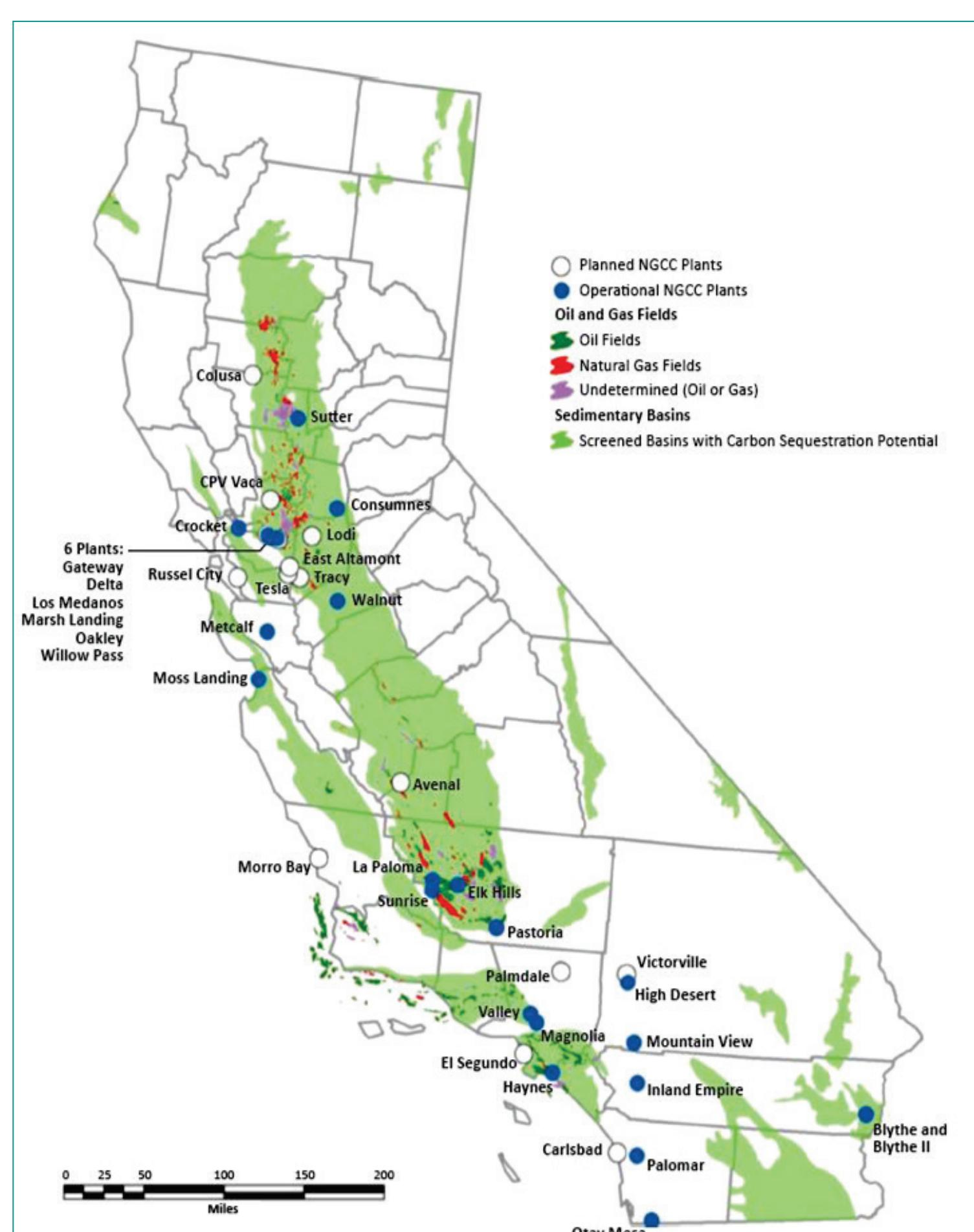
Many California NGCC plants (shown in blue and white circles) lie above or near sedimentary basins with CO<sub>2</sub> storage potential (shown in light green). CO<sub>2</sub> from NGCC plants could also be used for enhanced recovery operations in oil and natural gas fields (shown in dark green and red, respectively). Source: Lawrence Livermore National Lab and California Geological Survey
