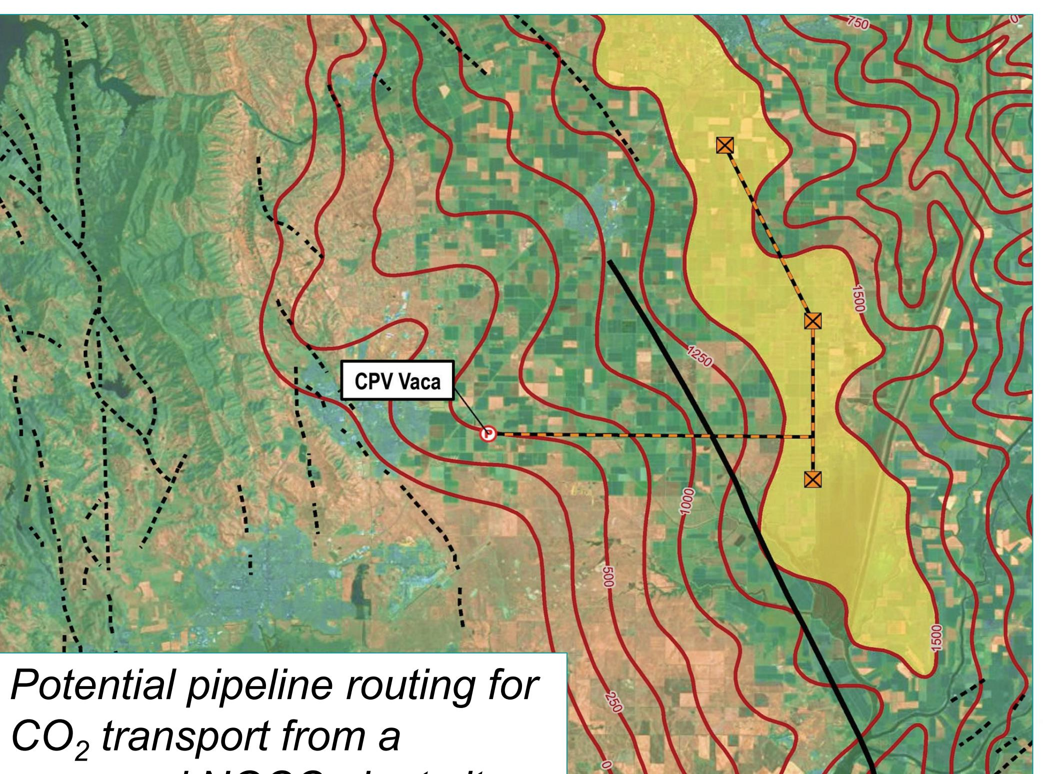
Potential pipeline routing for CO<sub>2</sub> transport from a proposed NGCC plant site near Vacaville, California, for injection into the thickest part of the Winters Formation (sandstone). Source: CB&I
