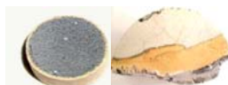
Experimental models (left) of cement integrity that correctly match field observations (right).
